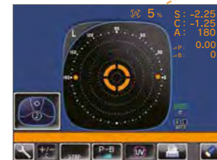
* UV Transmittance Measurement is performed with the light beam of 365 nm wavelength.
